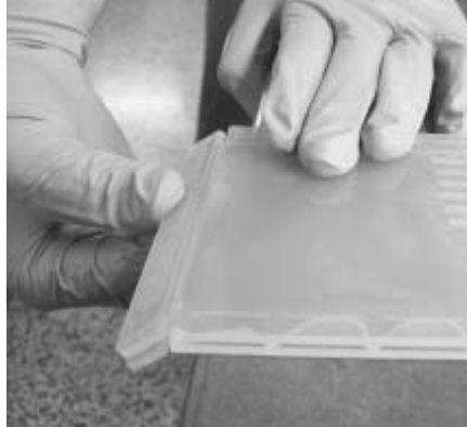
Figure 2. Removing the lower portion of the plastic cassette.
