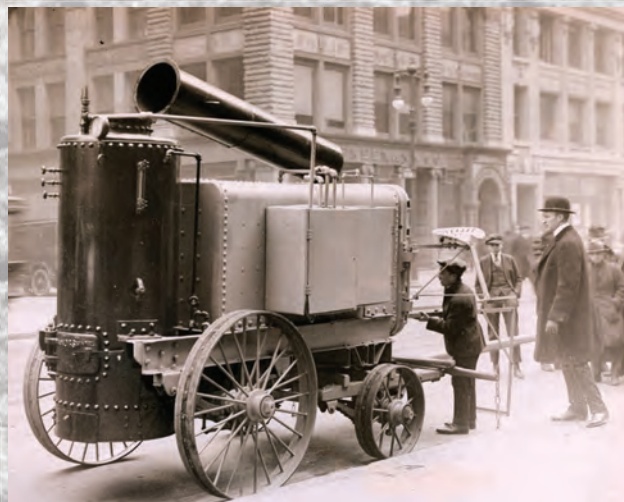
Lice that spread epidemic typhus were a serious concern on the front. This 8,000 pound steam sterilizer could kill those "cooties," as the soldiers called them, on the gear of forty men at a time.
